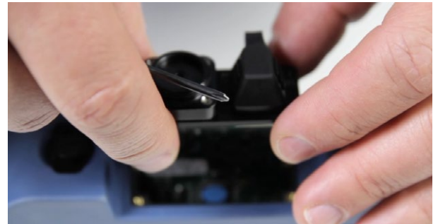
Figure 1. The power meter and VFL piece are offered as an easy-to-install option that's as simple as removing four screws.
