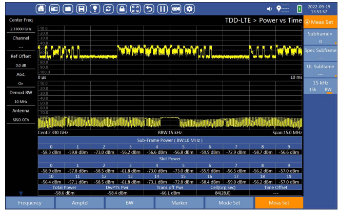
Figure 4: TDD-LTE power vs. time measurement.
